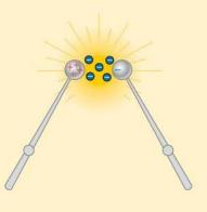
There is charge separation and nonzero potential difference  $\Delta V$  between the two spheres. The spark means that the air between the spheres becomes a conductor, leading to the rapid discharge and the production of light.
