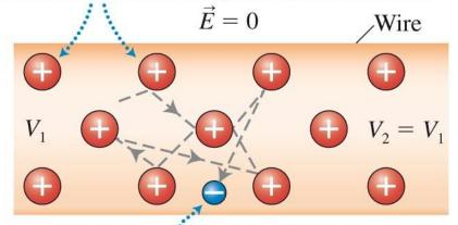
In the absence of an electric field, the electrons move randomly within the wire.
