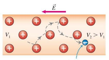
In the presence of an electric field, the electrons drift toward the higher *V* region.
