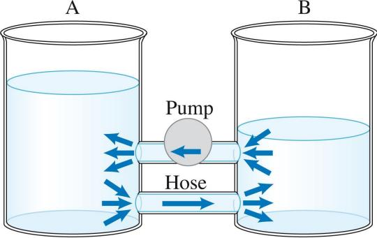
The pump returns water to container A. Water flows through the hose from A back to B.
