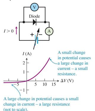
Using a diode in a circuit allows you to achieve onedirectional current.
