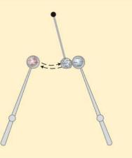
The foil ball must acquire a small amount of negative charge from the negative sphere each time it touches it. The ball carries the negative charge to the positive sphere and deposits it there and then returns to the negative sphere to repeat the process. This continues until the spheres are discharged and the potential difference between them is zero. The original electric potential energy is converted to mechanical energy and internal energy.
