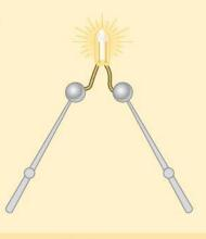
Before the bulb touches them, the spheres are charged and at different potentials. The bulb and its leads provide a conduction path to discharge the spheres. The discharge causes a flash of light from the bulb.
