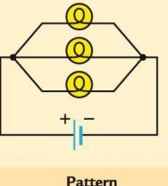
There must be an equal current through each bulb in every experiment, even when additional bulbs are added.
