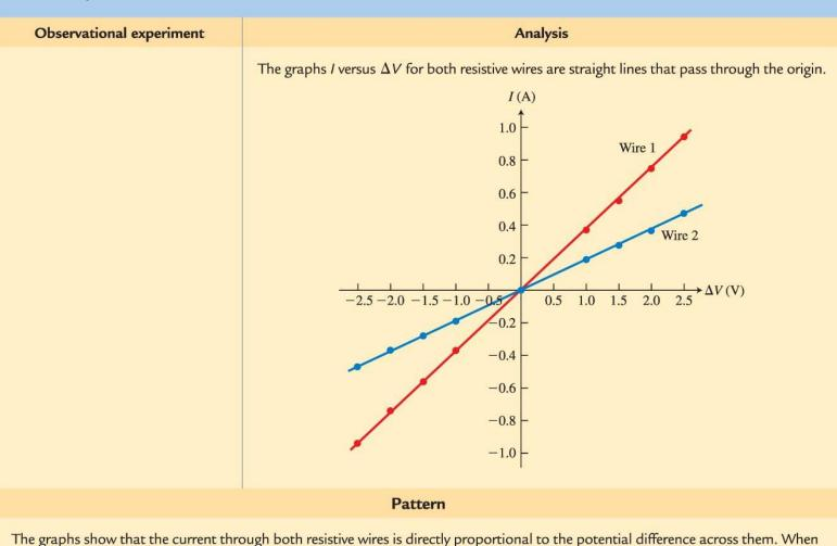
the potential difference reverses direction, so does the current. The slopes of the lines are different for different resistive wires.
